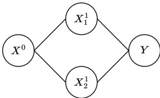
$$\vec{Z}^1 = \vec{w}^1 X^0 + \vec{b}^1, \quad \vec{X}^1 = \phi(\vec{Z}^1), \quad Y = \vec{w}^2 \cdot \vec{X}^1 + b^2$$
