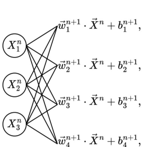
Diagram showing a fully connected layer with three input nodes  $X_1^n, X_2^n, X_3^n$  and four output nodes.
